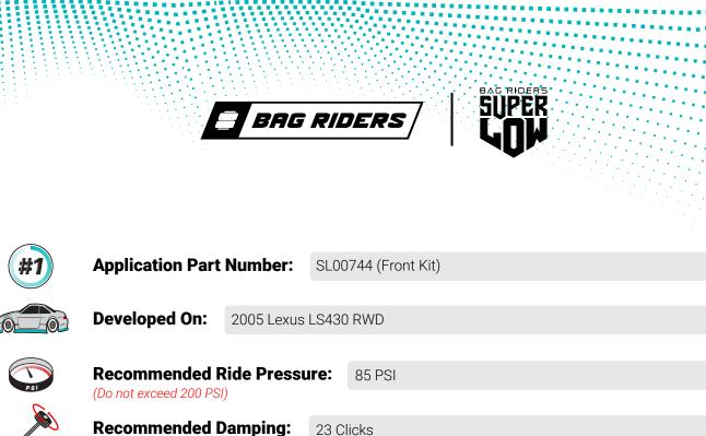
(Clockwise clicks from full soft) **Recommended Thread Length:** (Measurement between lockrings) 95 mm
